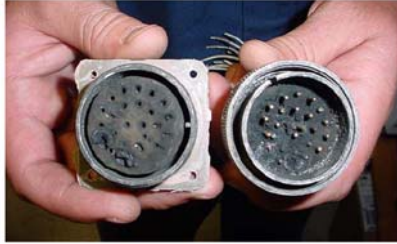
Figure 10.0 - P-3 flap well cannon plug shorted due to moisture intrusion and corrosion.
